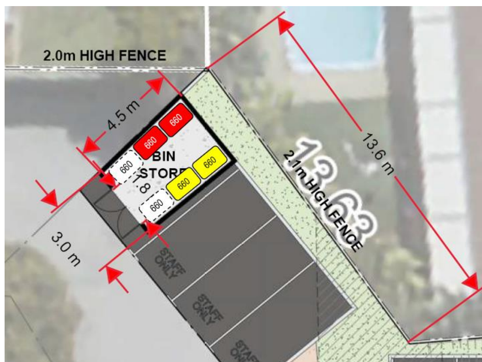
Figure 5 – Bin store showing space for up to six 660 litre MGBs and bin store dimensions (only 4 x 660L MGBs required)
