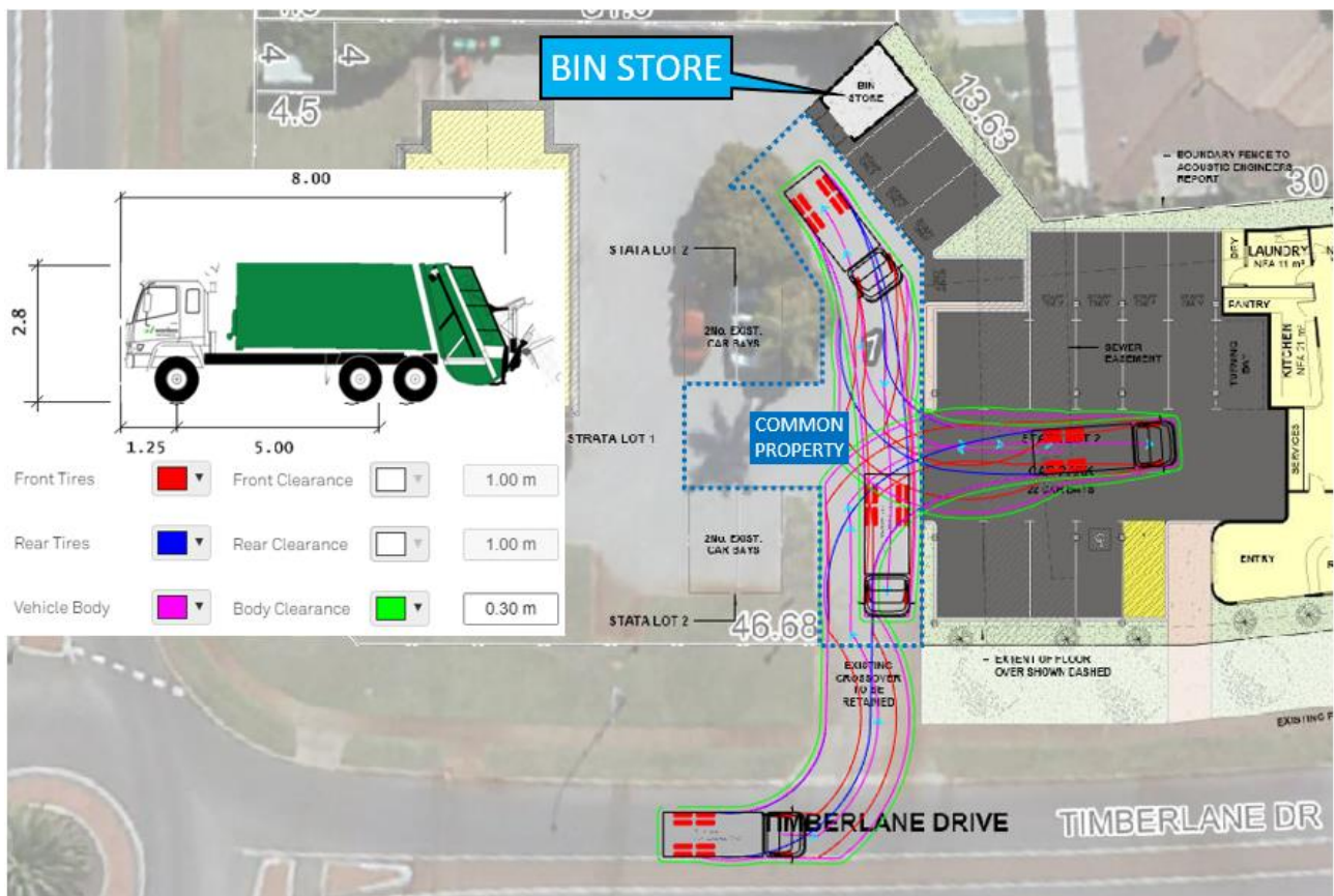
Figure 3 – Swept path of 8 m Waste Collection Vehicle and bin store location and service area
